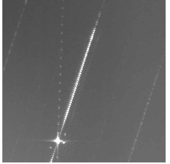
Figure 5. Fourier plane representation of the modulated signal from the SLM, showing that the signal is temporally broadband, repetitive, and that its source is located in the far-field of the antenna array.
